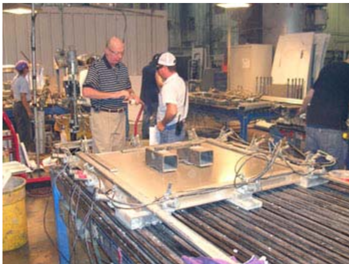
4-Star employees apply the adhesive to the trailer doors in preparation for the testing.
