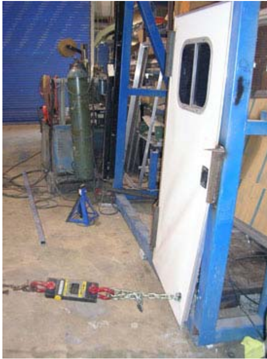
During 4-Star's testing, the adhesive withstood 1,600 lbs of force. Welds did not measure up.
